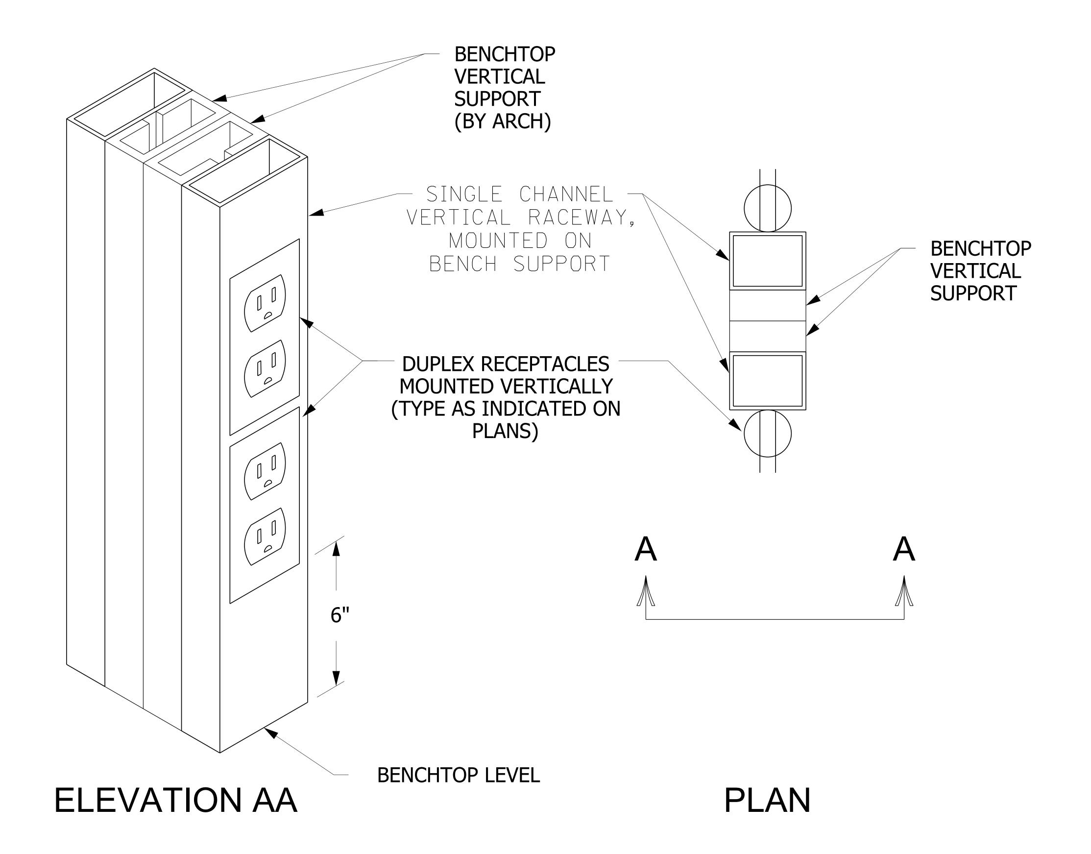
TYPICAL FOR ALL VERTICAL UNISTRUT ON BENCHES WITH DUPLEX RECEPTACLE SHOWN
